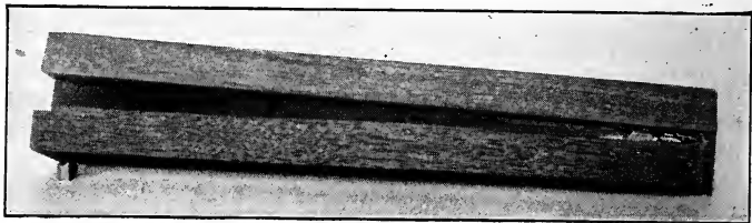
Fig. 326—Gluing up Column
